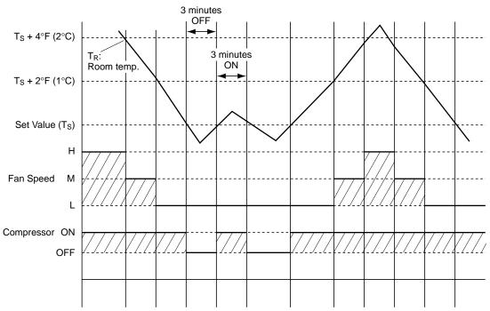
\* For 3 minutes after power ON, the compressor does not turn on.
